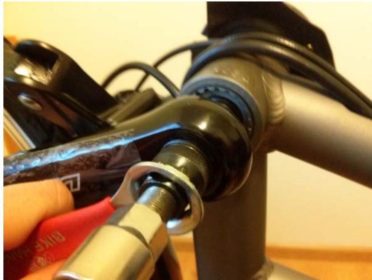
PLEASE NOTE: The shown above PAS sensor is not a standard component that comes with OXYDrive kits. Generally it should be fitted on the left arm to allow less complex installation of the kit.
