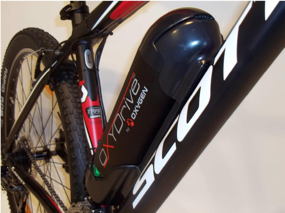
The battery holding unit should be fitted normally in the place of the water bottle cage. Most of the bicycles already have ready made frame decals where the water battery holding unit can be fitted.
