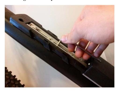
The battery holding unit should be fitted normally in the place of the water bottle cage. Most of the bicycles already have ready made frame mounts where the water battery holding unit can be attached to.
