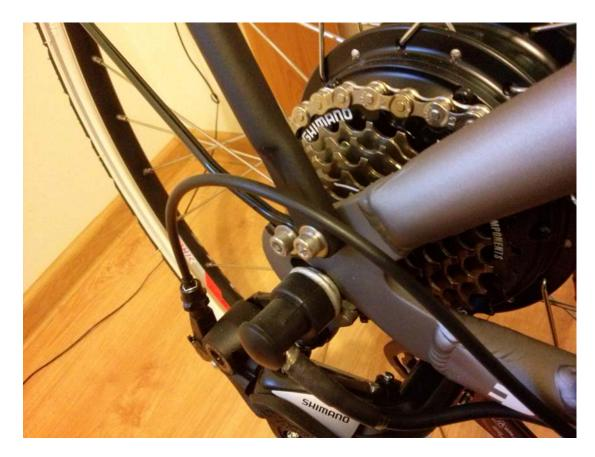
The battery holding unit with the rear carrier should be fitted to the frame mounts for rear carriers. Majority of frames have a special mounts where the rear rack can be attached to. Please make sure the bolts are well screwed in to the frame at it's full length of thread.
