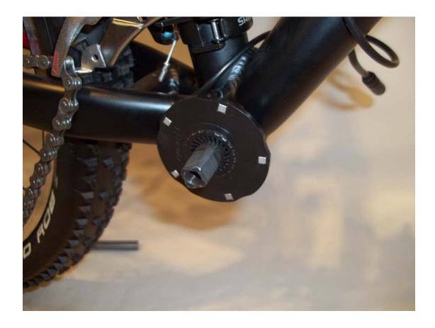
The magnet disc should be fitted on the axle with magnets located approx 1-3mm from the speed sensor.
