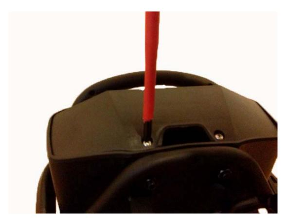
Open the lid from the controller compartment by using the screw driver
