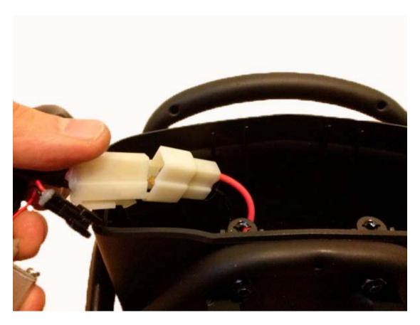
Connect the controller power connector with the battery connector. Connect other wires and slot in the controller in the controller box. Close the lid and fit the locking screws back again by using screwdriver.
